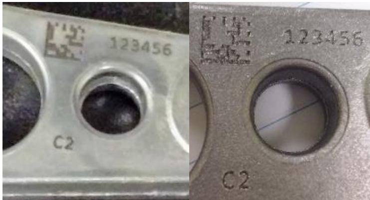
Figure 9: Photo of a marking before treatment (left) and after shot blast with S170 balls (center).
