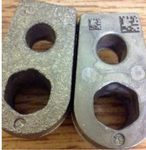
Figure 10: Photo of 2 samples after 20 seconds shot blast with S460 balls.
