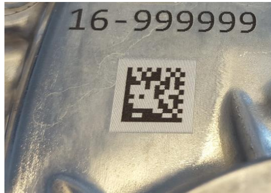
Figure 5: Laser marked identifier on aluminum die casting alloy.
