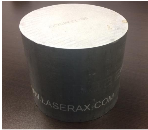
Figure 2- Laser marked identifier on a 3D surface made with a 3D head
