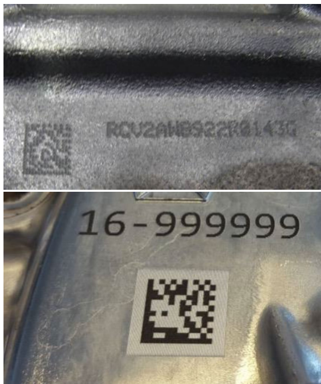
Figure 1 – Pin stamped (top) and Laser marked (bottom) identifiers on aluminum die casting.
