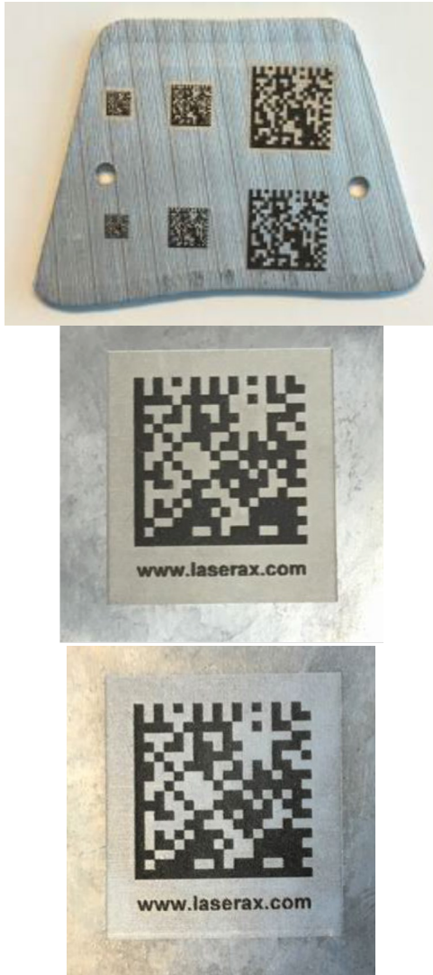
Figure 2 - Laser marks after chromate coating (top), and before (middle) and after (bottom) T6/T7 heat treatment.
